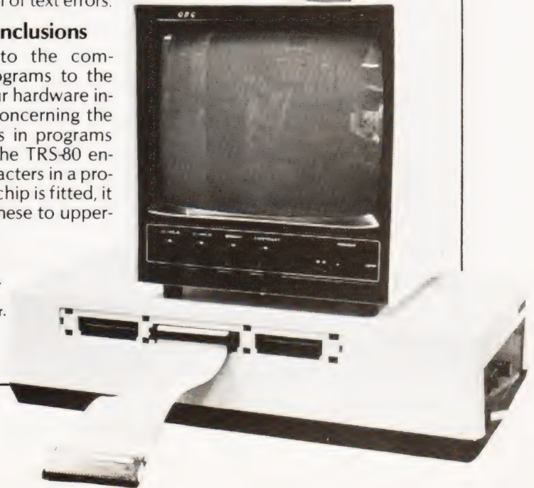
The expander and monitor units. Sockets are, left to right, disc, computer and Centronics printer.
